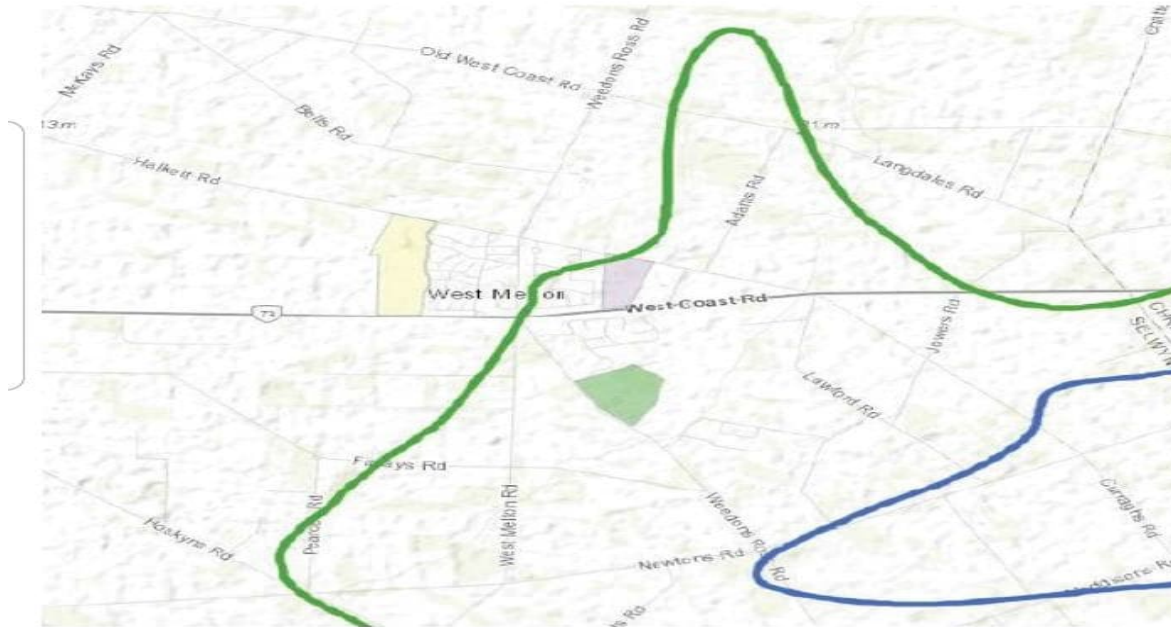
Map of proposed 50dB (green line) and 55dB (blue line) air noise contour, which encompasses some of West Melton, including the PC74 land (shaded area). Image: Supplied
