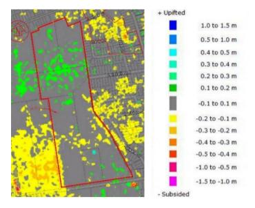
Figure 1 Lidar ground deformations, September 2010 to June 2011 Events
