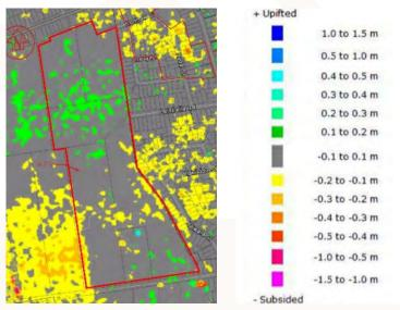
Figure 1 Lidar ground deformations, September 2010 to June 2011 Events
