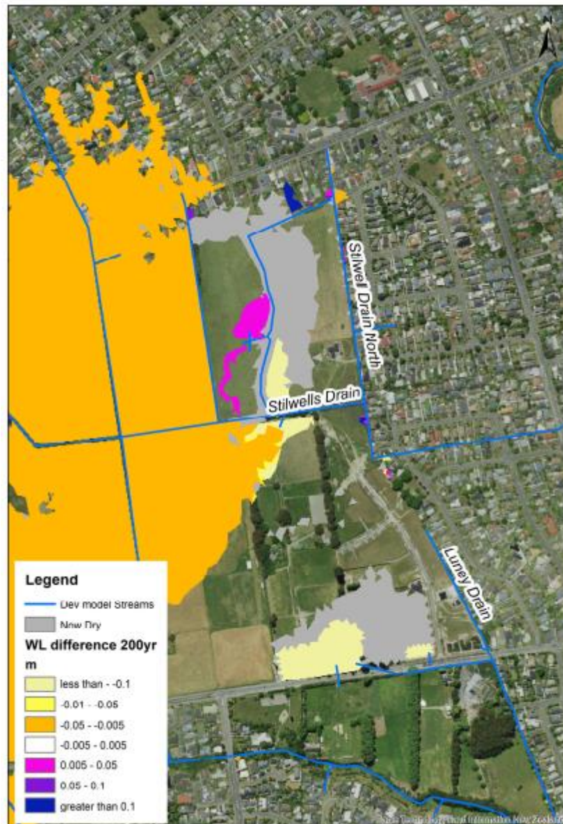
Figure 2 – Maximum water level difference, Development - Base
