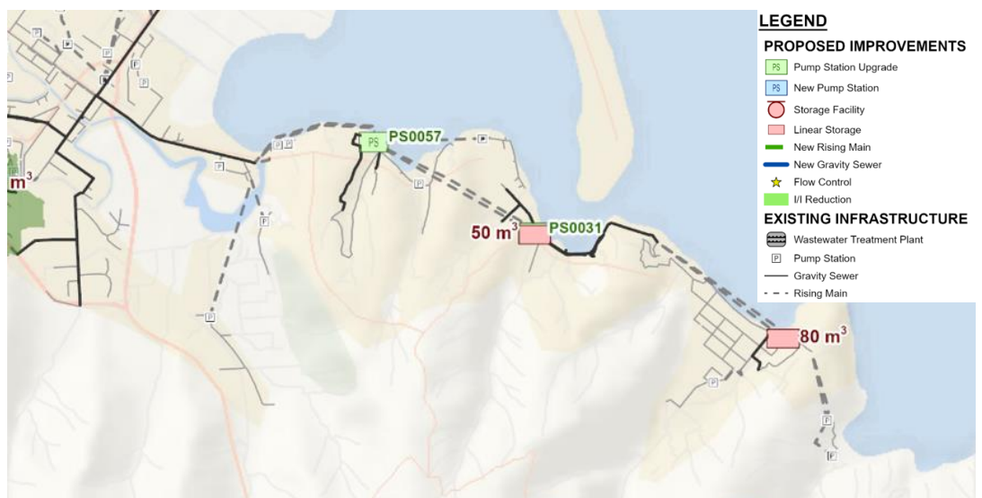
Figure 2 – Alternative solution to address current constraints and minimal growth in area east of Ferrymead Bridge
