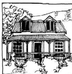
Verandah and simple gable with roof domers
