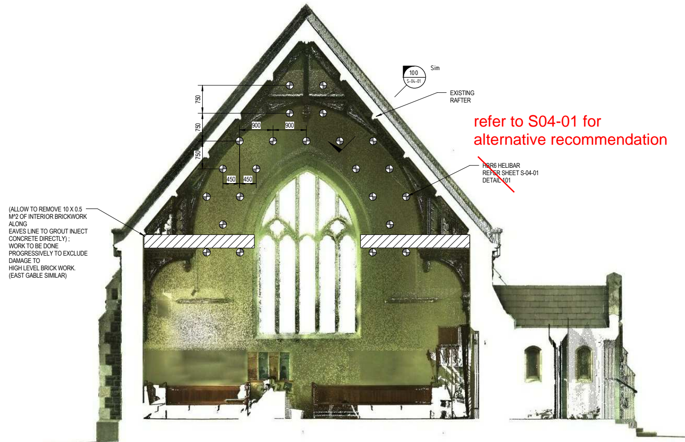
WESTERN WALL-INTERNAL ELEVATION (EASTERN WALL SIMILAR)
