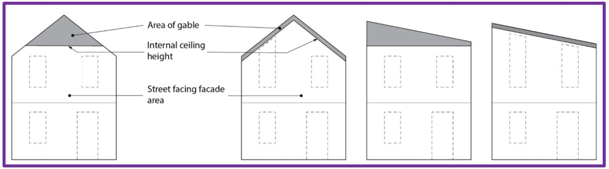
**Figure 3: How to measure street facing gable Example of different buildings with front gables excluded from calculation**
