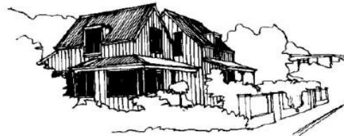
Multiple Gable Ends Roofs
