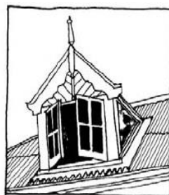
Dormer in a roof
