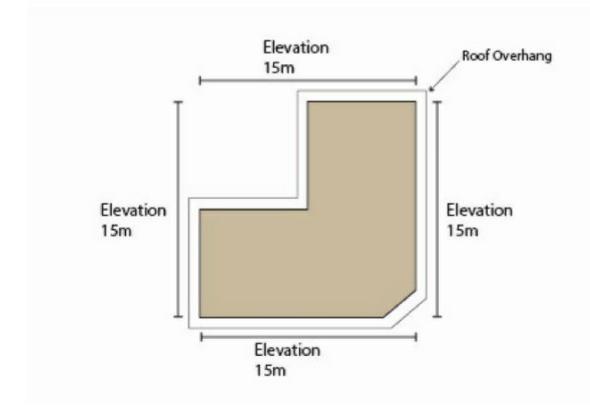
Figure 10: Measurement of a building elevation
