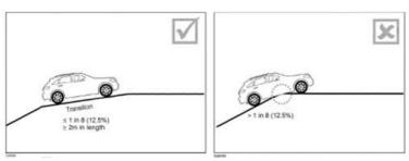
Figure 9 Example of correct and incorrect vehicle access gradient transition.
