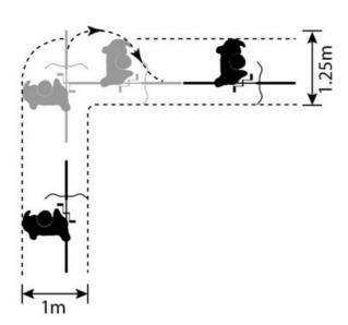
Figure 3 – Cycle turning circle - within the Central City
