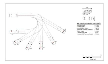
Figure 6-85 percentile design motor car
