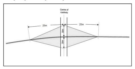
Figure 23 - Approach sight triangles for public road/rail siding level crossings.
