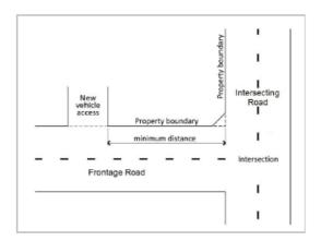
Figure 16 - Minimum distance of vehicle crossings from intersections outside the Central City
