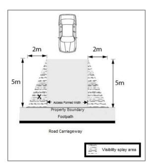
Figure 11 – Visibility splay measurement
