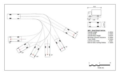
Figure 4 – Turning area for Small Rigid Vehicles
