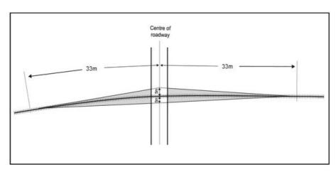
Figure 24 - Restart sight triangles for public road/rail siding level crossings.
