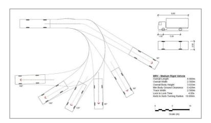
Figure 5 – Turning area for Medium Rigid Vehicles
