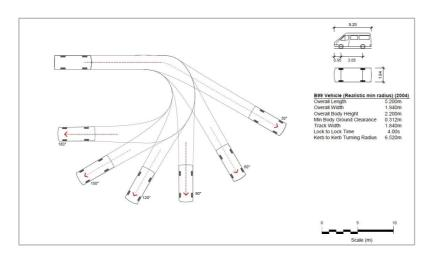
Figure 7 – 99 percentile design vehicle
