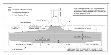
Figure 13 - Design of special use rural vehicle crossings
