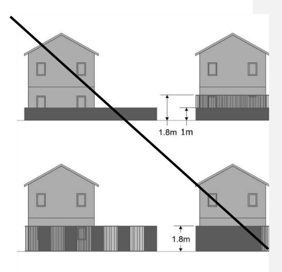
Figure 8: Examples of acceptable fencing and screening structures
