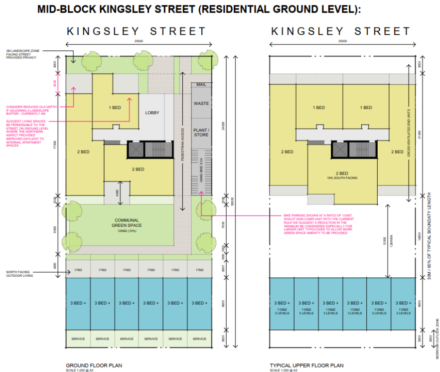
Figure 20 – Consultant testing of a ‘maximum residential’ scenario on a 25-metre wide site yields 34 dwellings (28 apartments and 6 terraces) with a RDA assessment for breaching the ground floor residential towards the street standard. Site yield is 190-dwellings per hectare.
