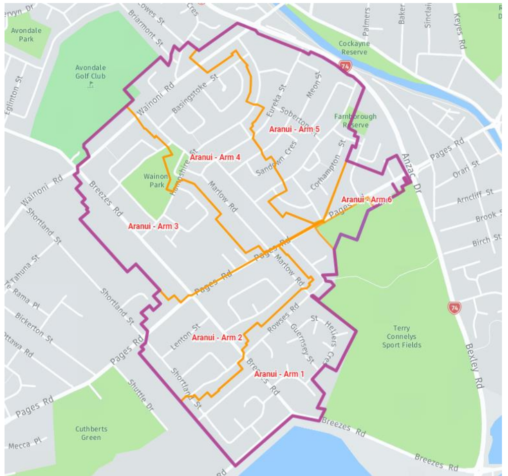
Figure 9 – Aranui Vacuum Sewer Catchment Layout
