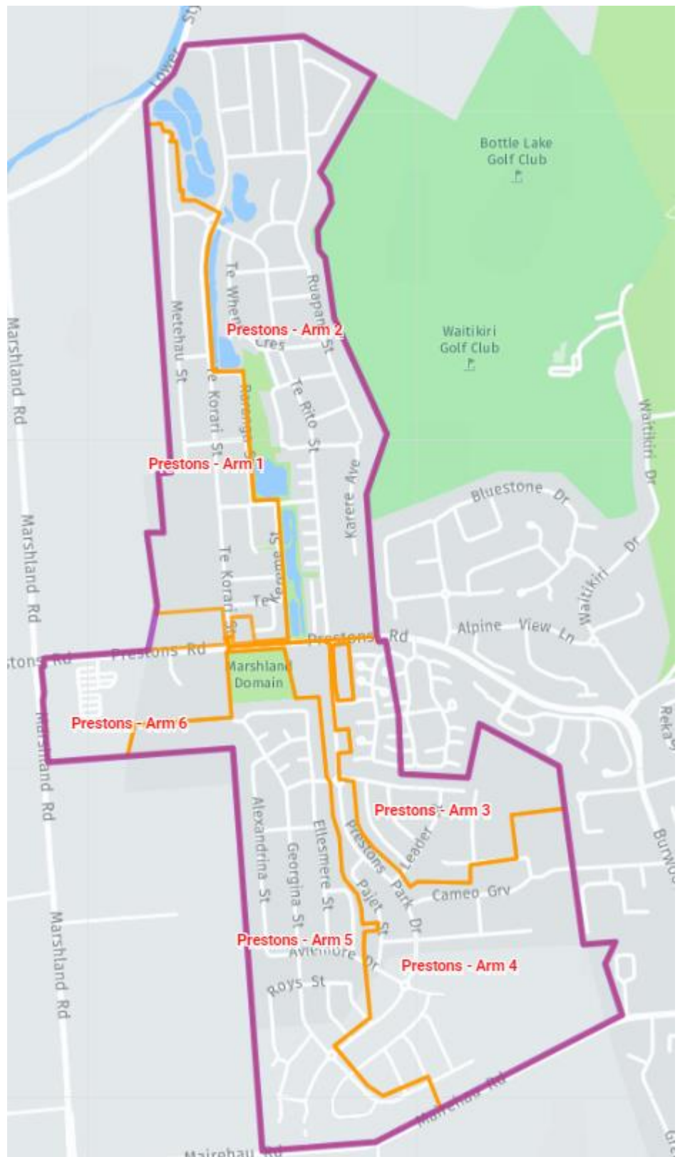
Figure 12 – Prestons Vacuum Sewer Catchment Layout
