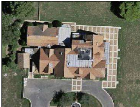
Aerial view of Daresbury (left). Note areas of metal trough roofing and well in centre of the roof. Roof tiles (right). Note scalloped tiles and crested ridge tiles.
