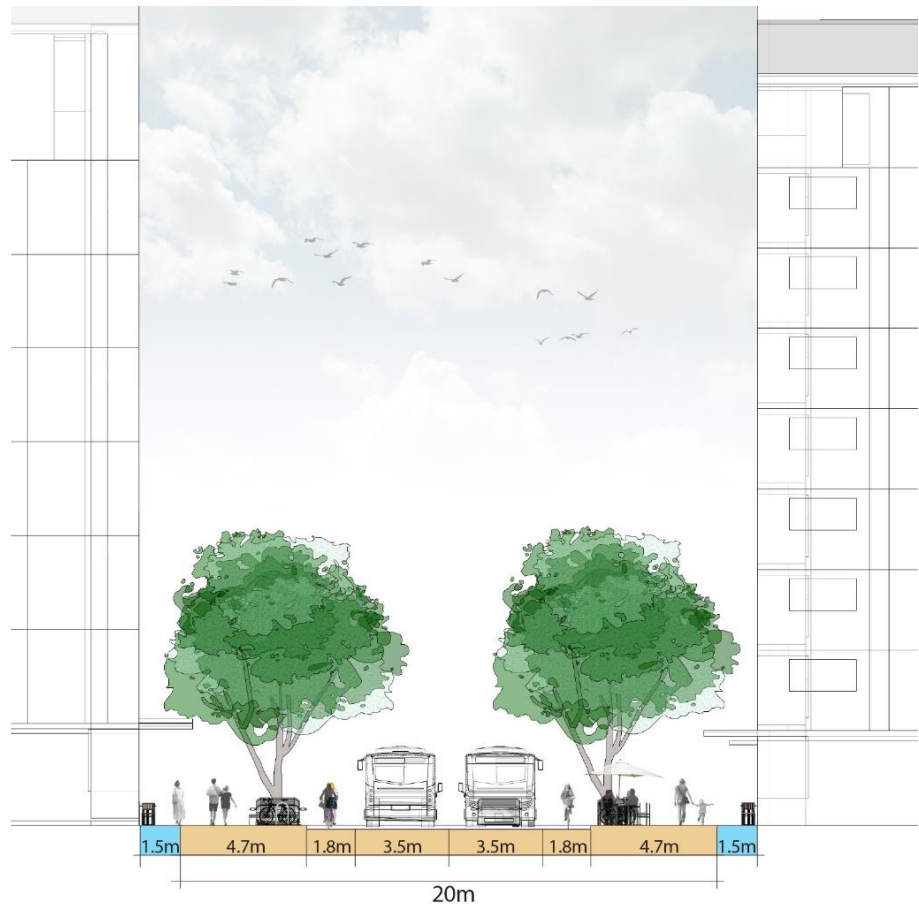
Figure 5 – Typical cross-section showing a 20m wide commercial ‘Main’ street with a 1.5m setback. (NTS)
